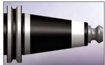
The marks at the gauge line and at the threaded area of the toolholder shanks started to show up after the retention knob was used rather than the draw bar. The area between the gauge line and the threaded area have no marks. The tolerances of the toolholder tapers were suspected as the cause of the marks. In response, the tool manufacturers tightened the grinding tolerances from .000130 inch to the AT3 limit of .000079 inch, but the marks on the toolholder shanks are still present today.
