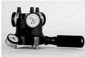
J&M Machine used the Taper Shank Test Fixture to test different retention knobs and toolholders on the market and was able to prove that standard retention knobs made to any of the 5 world standards expand the toolholder shank at the small end when tightened to an adequate torque pressure to preload the knob.
