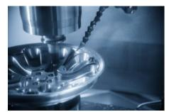
The CNC milling machine or machining center cutting the mold part. Injection mold insert making by CNC machine.
