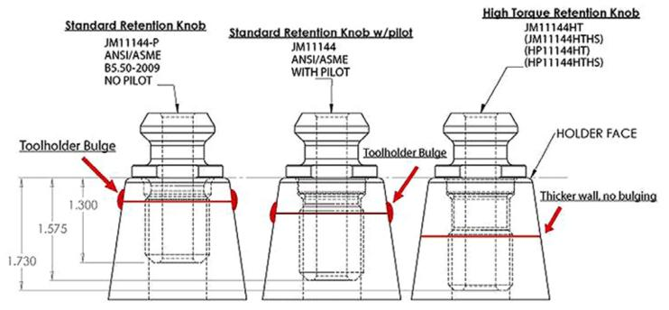
JMPP's high torque retention knobs overcome a key design flaw inherent in CNC v-flange tooling, eliminating the toolholder expansion responsible for costly CNC milling and boring issues.
