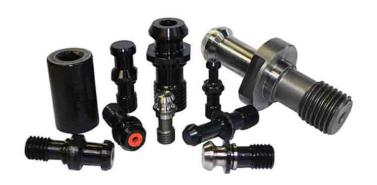
The High Torque retention knob is designed with a longer reach, so that it threads deeper into the threaded bore of the toolholder. Consequently, all thread engagement happens in an area of the toolholder where there is a denser cross-section of material to counter deformation.
