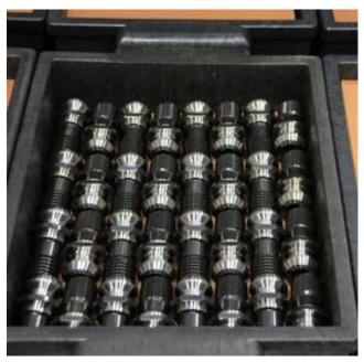
A series of retention knobs in a case. The High Torque retention knob includes a precision pilot to increase rigidity, and is balanced by design. Photo courtesy of JM Performance Products.
