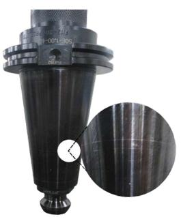
After-use images of standard vs. high-torque retention knobs. The first image shows taper deformation which prevents a toolholder from properly mating with the CNC machine's spindle. The second image reflects high-torque retention knobs' design elements that improve taper contact close to 100%.
