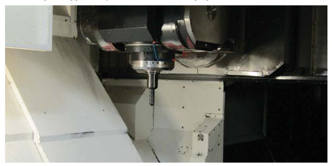
Campos says improvements on HEC's Mazak 5-axis CNC machining center, featuring 160" length with dual shuttle tables and a tool-changer designed to run one table full of parts while the other is being loaded. "Our Mazak machines used to make a loud noise when changing tools, and JMPP's high-torque retention knobs solved that problem," Campos says. "The machines are much quieter now when roughing titanium and stainless steel. They also eliminated fretting of the toolholder shank."
